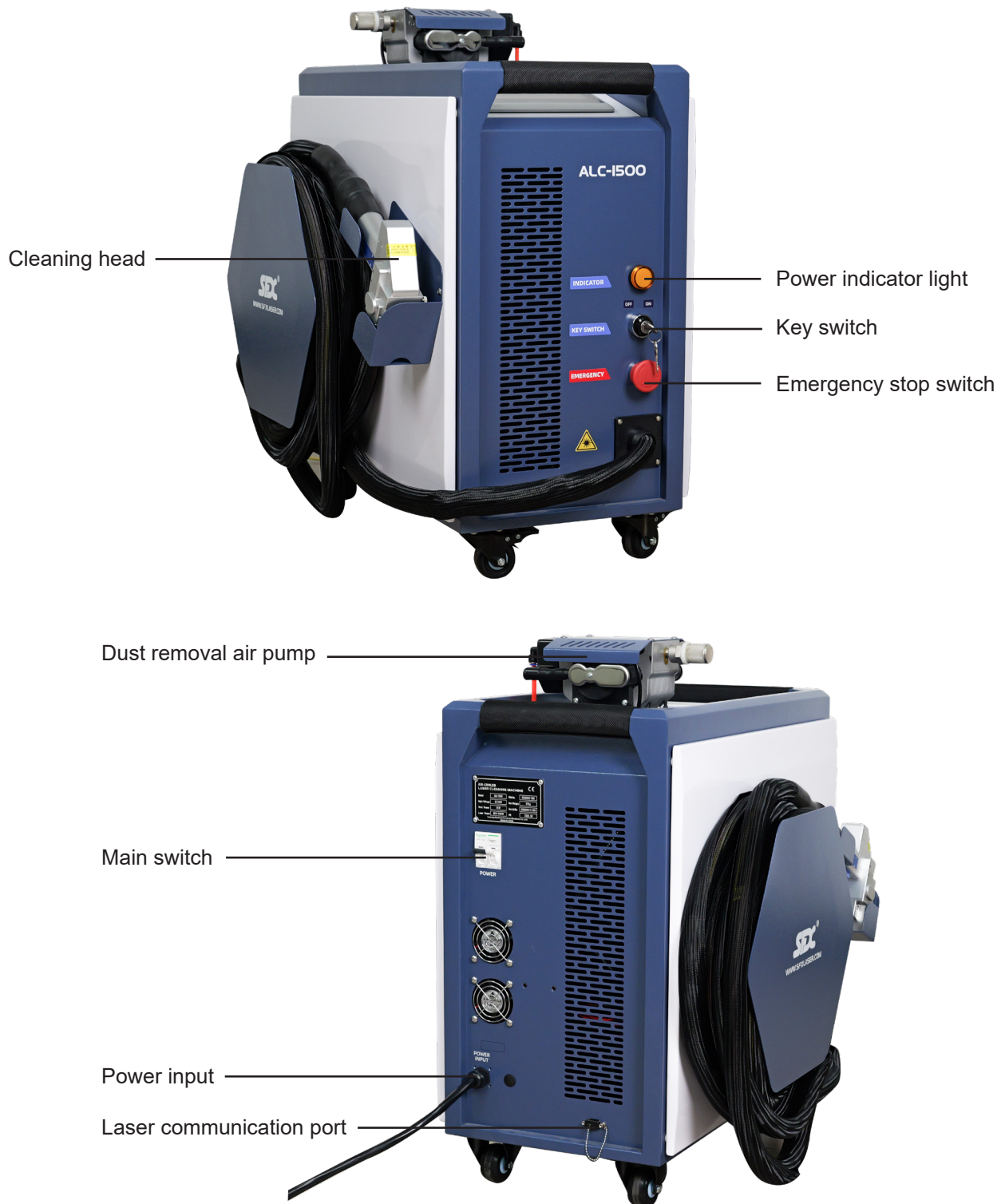
Figure 1 ALC-1500 structure diagram
